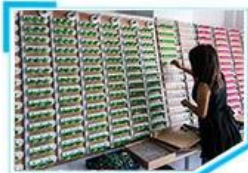
9. Aging test for travel charger
