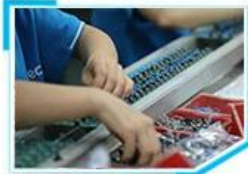
5. Plug in components and parts
