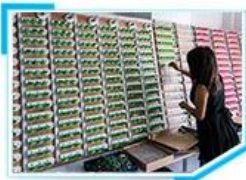
9. Aging test for travel charger
